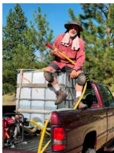
COURTESY OF CHRIS BIRCHMAN Chris Birchman’s Dodge pickup is equipped with tanks, pumps, and hose to take the water wherever it might be needed on his property.
