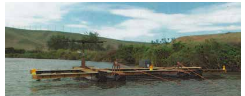
COURTESY OF WDFW The WDFW PIT barge measures 15 feet wide by 28 feet long. Extended arms increase the width to about 40 feet.
