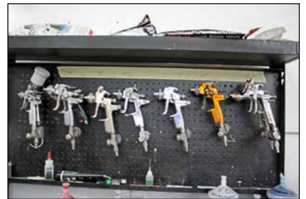
Tools of the trade. Many types of paint "heads" are needed depending on the vehicle, type of paint and style desired.
