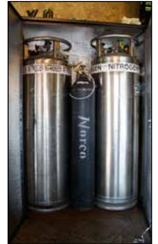
Liquid nitrogen tanks
