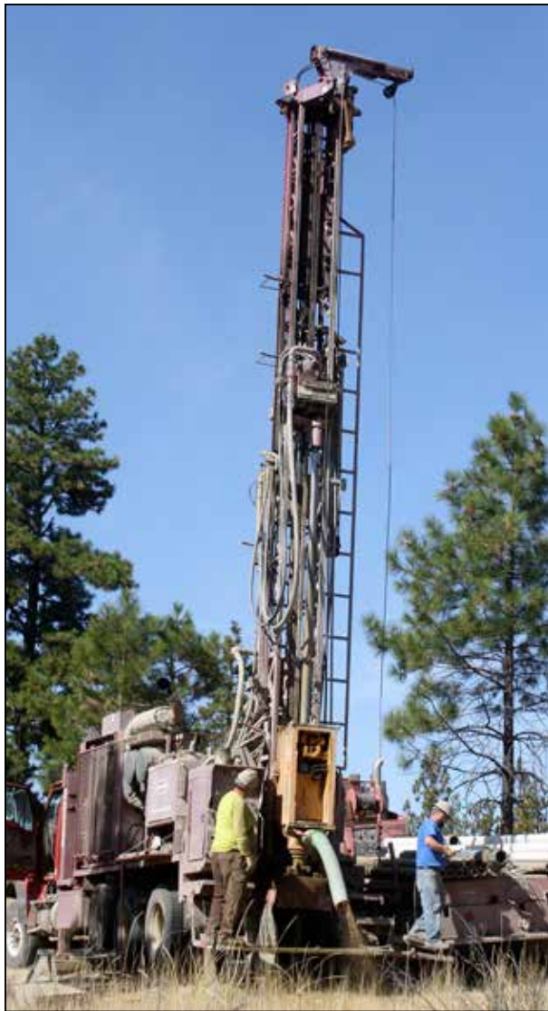
The top-heavy drilling rig must be leveled before any drilling can begin.
