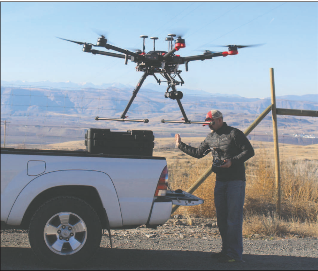
CLOCKWISE FROM LEFT: Erlandsen’s drone takes flight along Cameron Lake Road. Jesse Revel programs and monitors the drone flight from his laptop. White-capped GPS sensors coordinate the drones positioning. The gimbal-mounted camera can be replaced with other devices like a thermal sensor.
