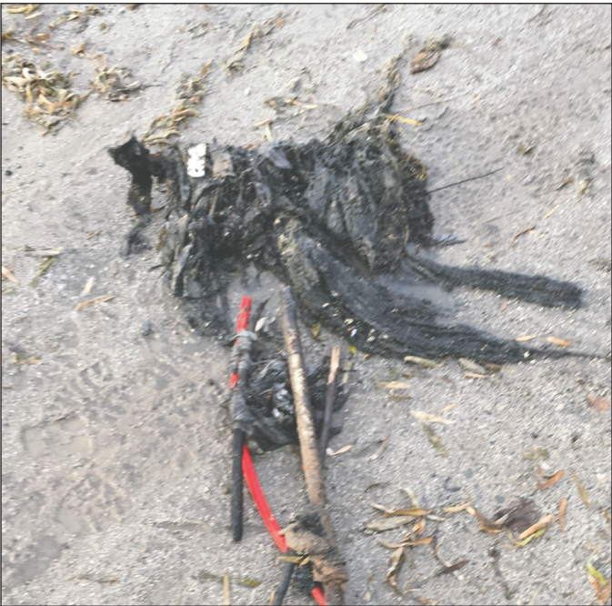
Photo courtesy of Lee Webster This attention-grabbing glob comprised of flushable wipes and some tubing pulled from a section of city sewer line was about the size of a five-gallon bucket.
