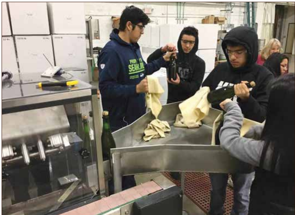
Photos courtesy of Chelan High School's Facebook ABOVE: Viticulture students worked the sparkling wine bottling like at Karma Vineyard's processing facility in Entiat. The wine is fermented in the bottle with the yeast and then the yeasts gets removed in this process, the machine helping put in the final cork to the highly pressurized liquid. BELOW: Students in Viticulture braved the cold along the Columbia River by removing grow tubes from young grape vine plants. The grow tubes protect the young vines from critters and from farm equipment, as well as holding in moisture and warmth.
