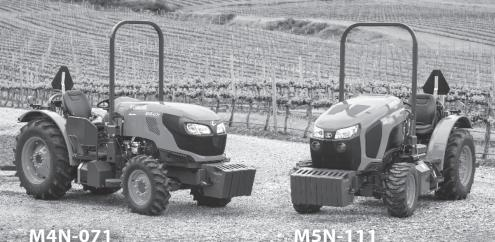
Take on vineyard and orchard work with three powerful horsepower options, versatile 12 or 24 speed transmissions, hydraulic shuttle, Bi-Speed turning, wet disc brakes and more! Open station and cab models available!
