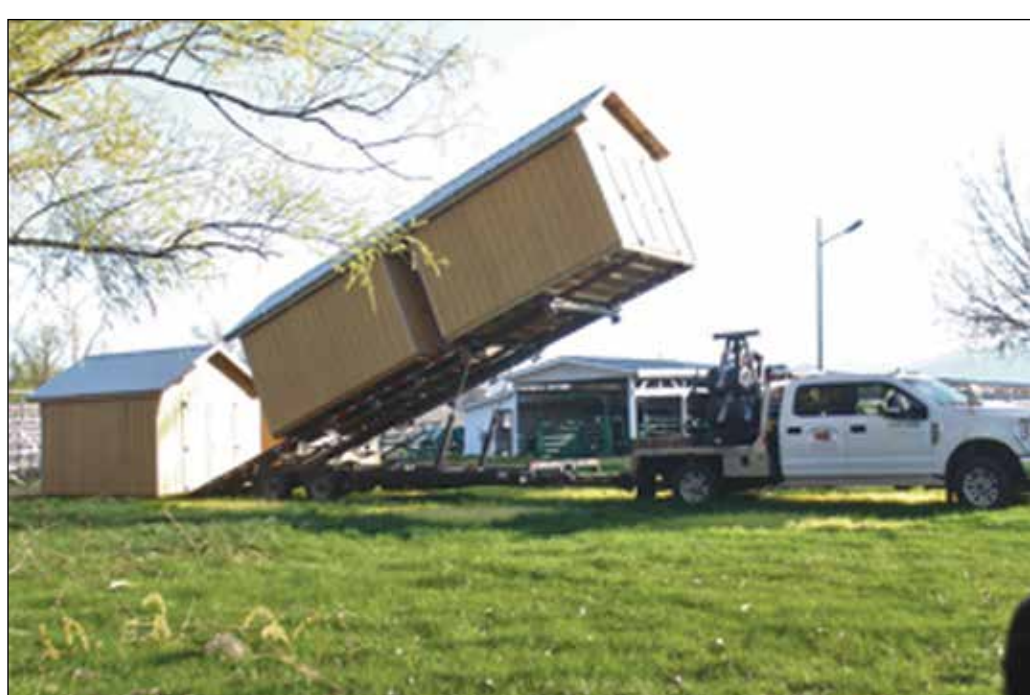
Yoder loads a trio of 8-x-12-foot sheds on his hydraulic tilt trailer before heading out to make deliveries from Palmer Mountain in Okanogan County to Pearl Hill in Douglas County.
