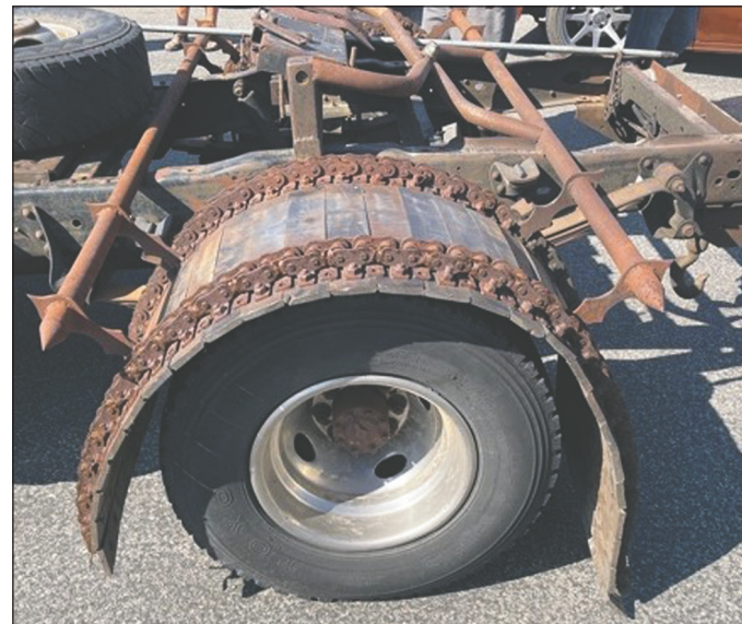
Mill conveyor belt fender.
