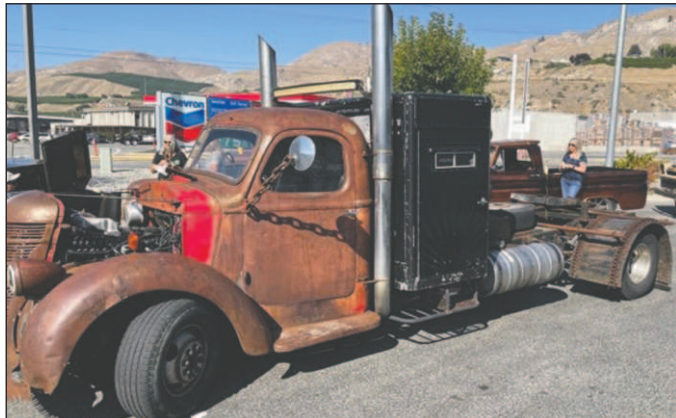
Aaron Post's 1937 International truck displays unique touches like a crosscut saw bumper, mill conveyor belt rear fenders, and welded links of heavy chain for mirror arms.
