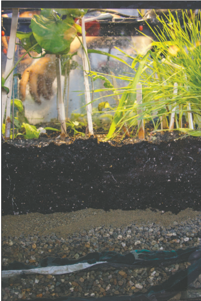
Each tank included soil layers consisting of a gravelly loam layer, a gravelly sand layer and top soil.
