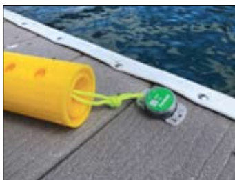
Bella Gatzemeier and Phil Long of the Lake Chelan Research Institute check the #D printed solar shield and temperature sensor design for deployment at Peterson's Waterfront near downtown Chelan on June 29. BELOW: A closeup of the #D printed solar shield and temperature sensor design.
