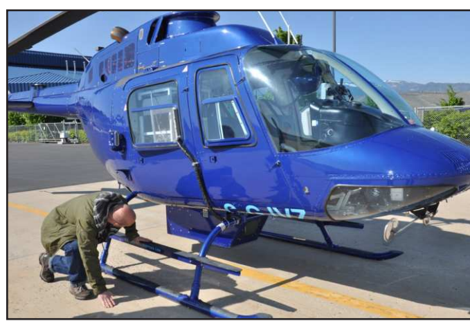
Photo submitted by Kimberlee Craig Chelan PUD's contractor prepares to fly over sections of transmission line with specialized laser equipment to capture data for mapping and to analyze reliability.
