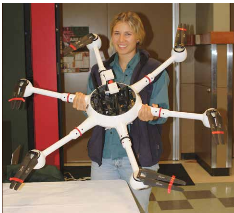
Consulting Group Area Coordinator Natalie Rodriguez holds a drone that can be used to drop sterile Codling Moths on orchards.
