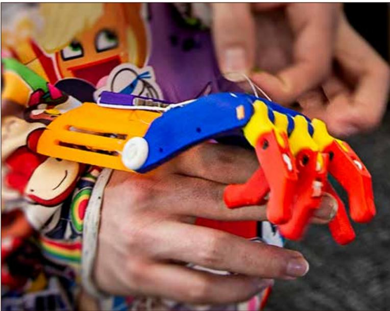
3D printers can make pieces of complex tools, like this prosthetic hand created and assembled by CHS sophomore, Collin Stitt.
