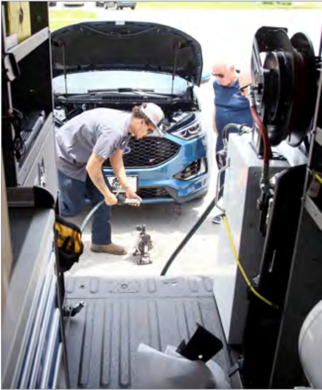
Jim Baier technician Derion Scully hooks up an oil reclaimer to a pump before changing the oil on a Jim Baier vehicle Wednesday afternoon. The service is part of Jim Baier Ford's new Mobile Service Van that will be put into service next week.
