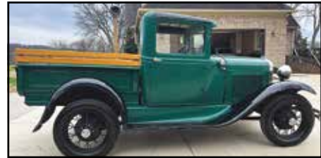
1931 Ford pick-up (completely restored, 4 cylinder, 3 speed)
