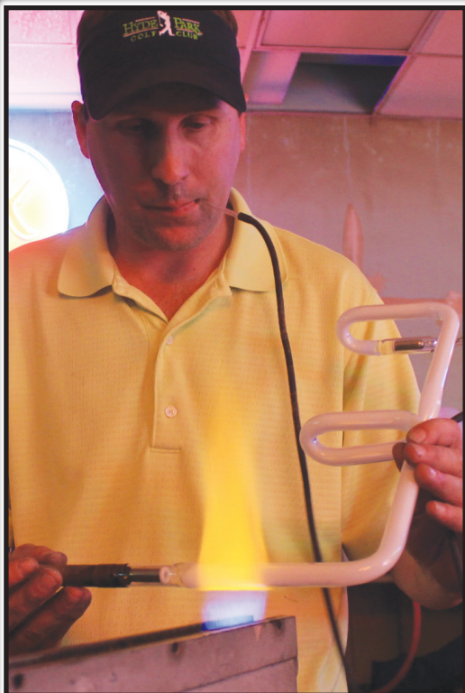
Melting glass and bending it. Chris Petney uses a 700-degree flame to melt the glass while he blows into the tube so he can bend it into its desired shape.
