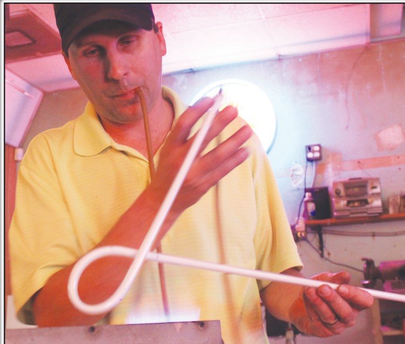
Melting glass and bending it. Chris Petney uses a 700-degree flame to melt the glass while he blows into the tube so he can bend it into its desired shape.
