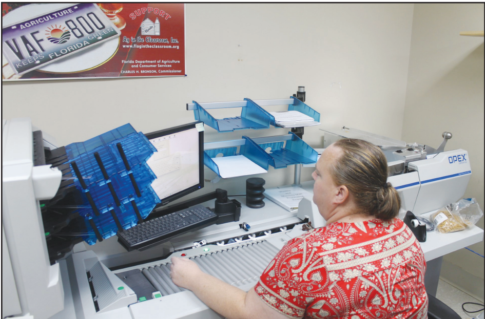
A Tax Collector staff member shows how a machine can open, sort and catalog envelopes with checks to be deposited. The process saves hours of valuable time - and money.
